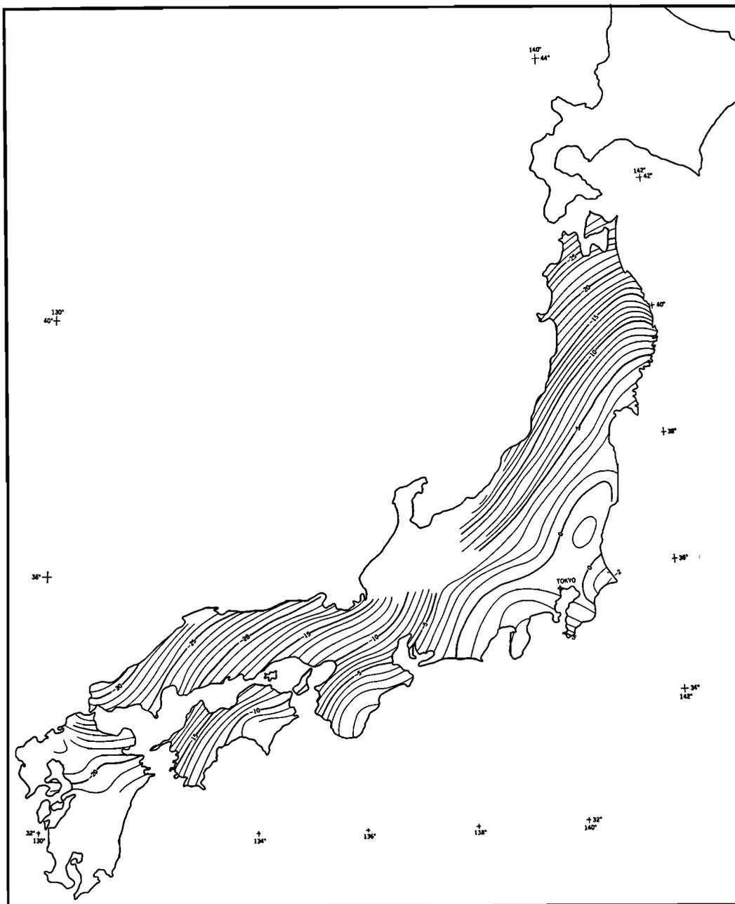
FIG. 8—Japan, geoidal contours in meters, Tokyo Datum
