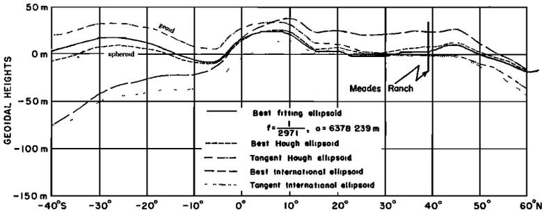
FIG. 5—Geoidal heights relative to various ellipsoids, America, 100th meridian
