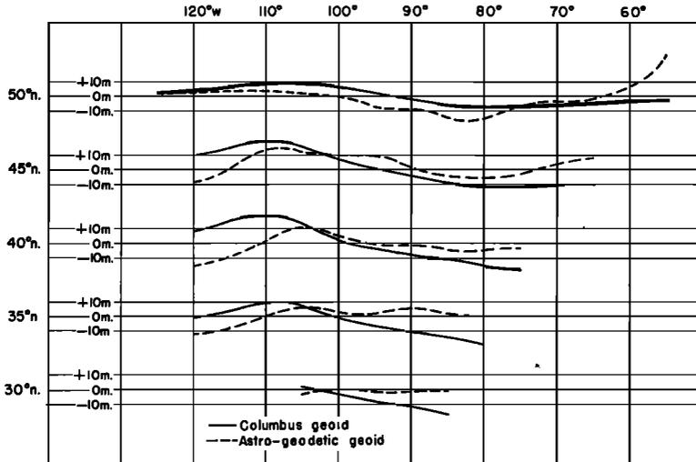
FIG. 12—Columbus Geoid in America, profiles along parallels
