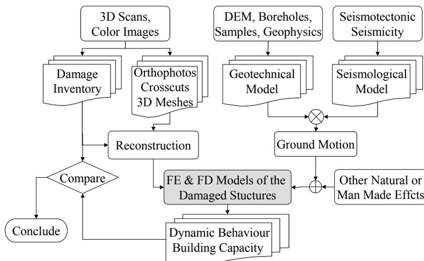
Fig. 1: Schematic flow chart of quantitative archaeoseismic modelling.
